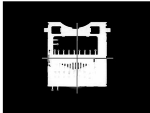
Caption: Back light recognition is ideal for odd-shaped components
