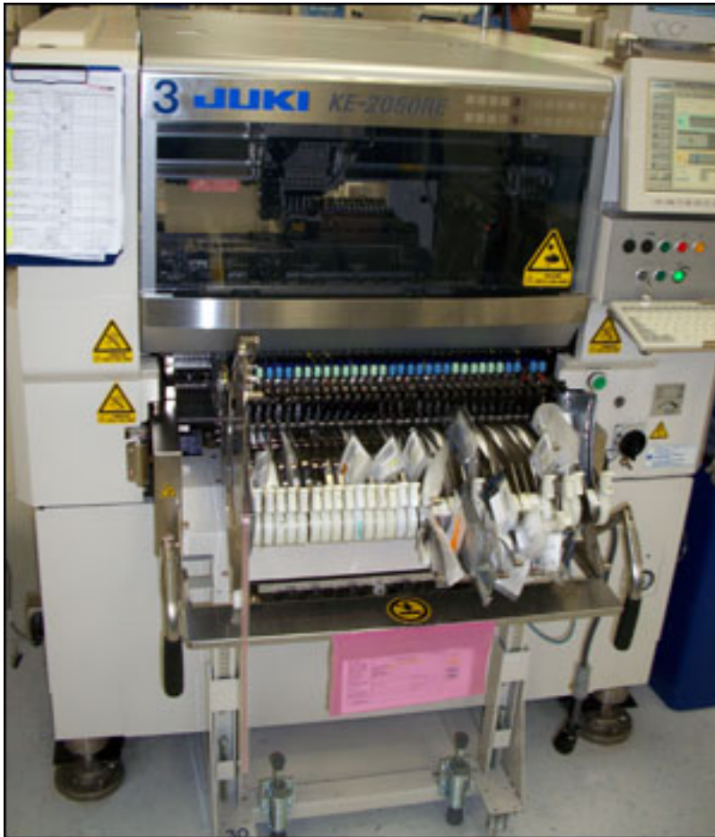
When a trolley is inserted into a circuit-board assembling machine, the system uses RFID to verify that all the feeders and reels are still in the correct position.
