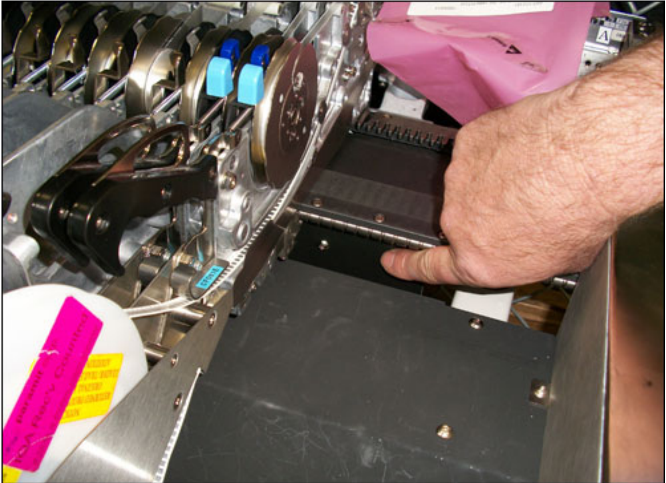
Each of a trolley's feeder slots has an RFID antenna.
